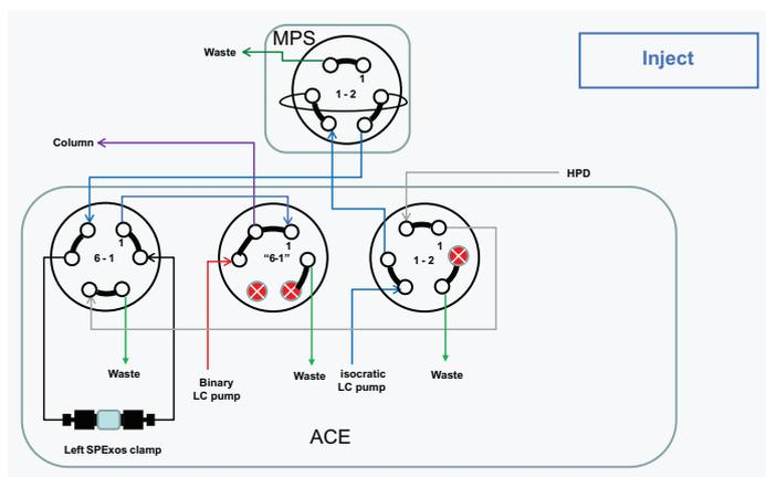
**Figure 2:** Flow diagram showing valve settings during injection: Elution of the cartridge with ammonia in methanol going through the injection loop, merging with formic acid in water in the T-rotor valve (middle).
