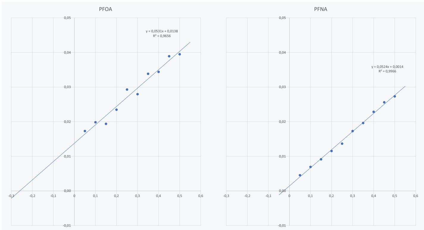
Figure 8: Example calibration curves in the range 0.05 – 0.5 ng/L with and without significant blank.
