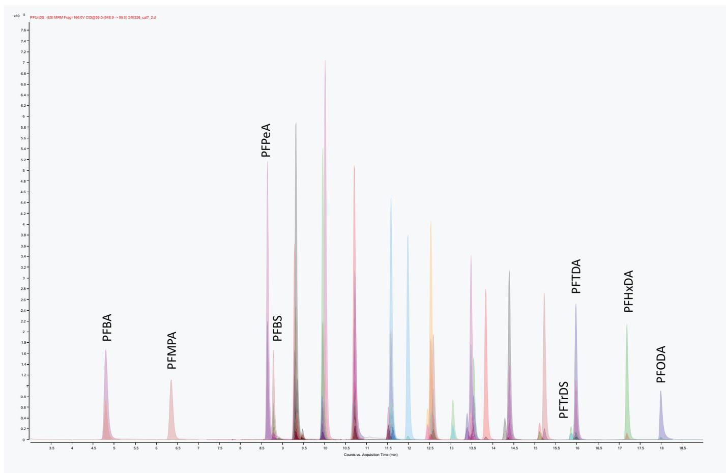
**Figure 3:** Example chromatogram for a standard solution (50 ng/L) in water with all recorded MRMs, first and last eluting peaks are annotated.
