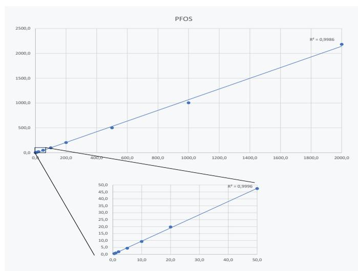
**Figure 5:** Example calibration curve in the range 0.5 – 2000 ng/L (enlarged area 0.5 – 50 ng/L).
