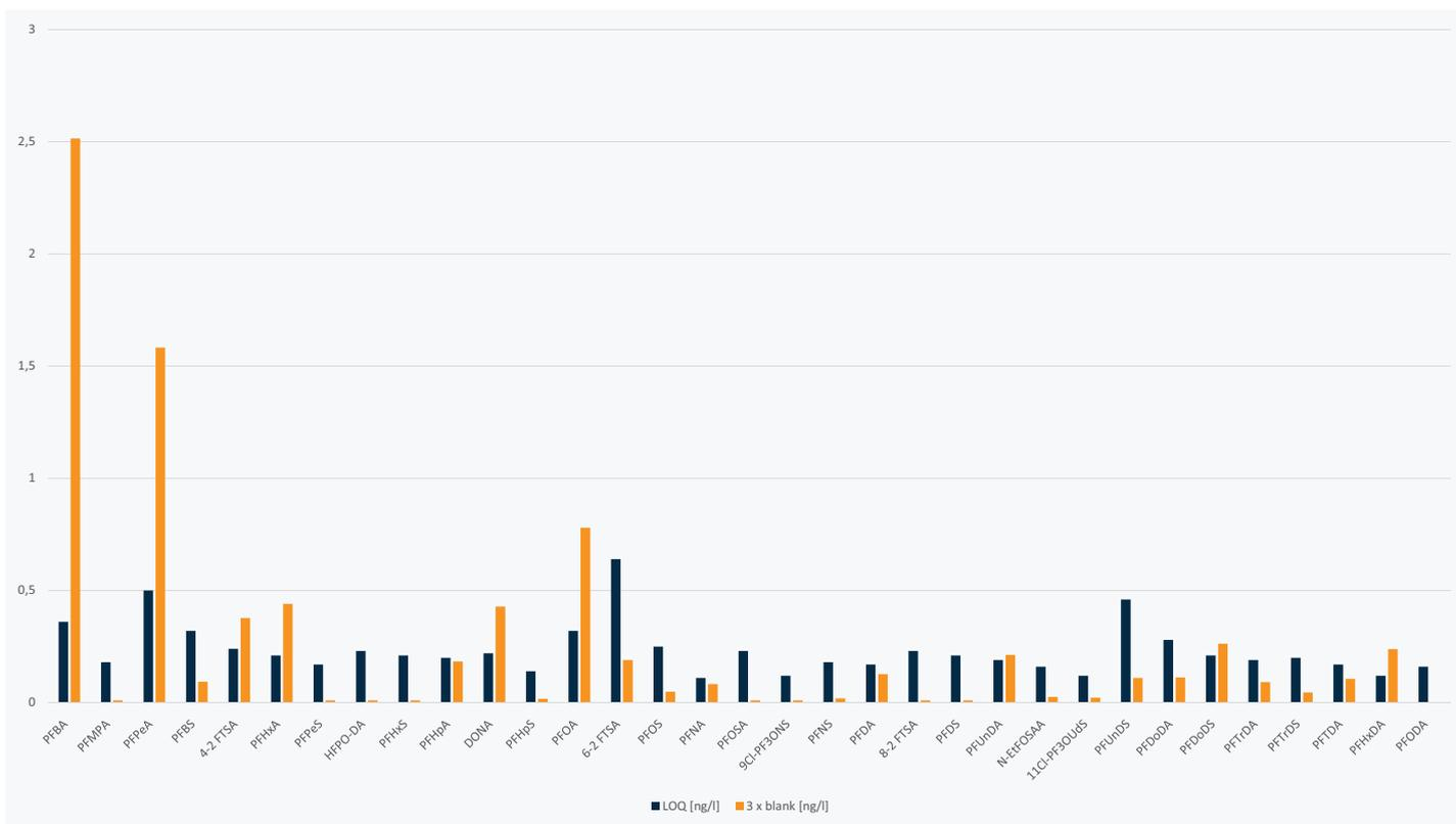
Figure 9: Limits of quantification compared to the blanks calculated from calibration curves in the range 0.05 – 0.5 ng/L.
