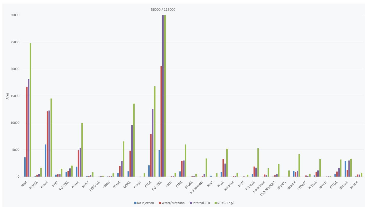
**Figure 4:** Blank determination and comparison with a low level calibration standard (0.1 ng/L).
