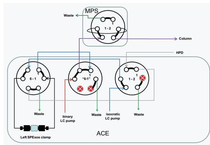
**Figure 6:** Modified system for the determination of recovery rates by direct injection onto the column under online-SPE conditions.
