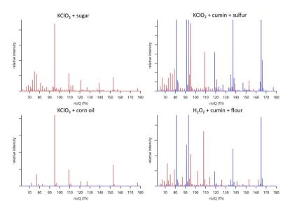
*Figure 4* Chemical fingerprint of potassium chlorate and concentrated hydrogen peroxide mixtures. Note the characteristic molecules at 95, 109, 121, 139, and 153. In the mixtures including cumin, the molecules derived from the cumin are highlighted in blue.
