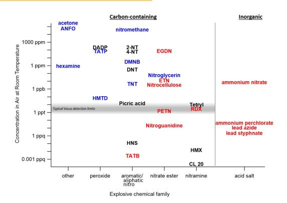
**Figure 1** Explosives and related chemicals arranged by volatility and chemical structure. Compounds with proven detection by Vocus CI-TOF are shown in blue, untested compounds in black, and undetectable compounds in red. Typical Vocus CI-TOF detection limits with 1-second measurement are indicated by the gray shaded area. The volatility of lead azide and lead styphnate is unknown but likely low.
