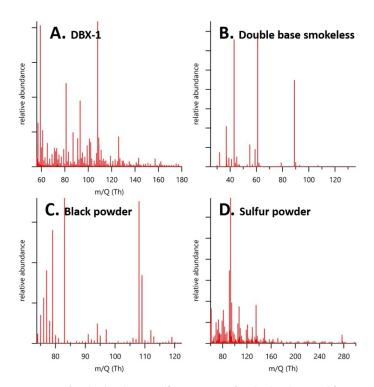
**Figure 6** A) Volatiles detected from DBX-1. B) Volatiles detected from double base smokeless powder. The largest signals are related to organic acids and ethyl acetate. C) Volatiles detected from black powder. D) Volatiles detected from sulfur powder.
