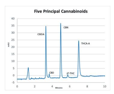
UV detection of five cannabinoids at 255 nm using the Axcend Focus LC. Elution Order - 3.3 min: CBDA; 3.6 min: CBD; 5 min: CBN; 5.8 min:  $\Delta$ 9-THC; and 7 min: THCA-A. Flow rate: 3  $\mu$ L/min; Gradient: 65% - 85% B, 10 min; Equilibration Time: 2 min; Mobile Phase A (3:97:0.1 acetonitrile [ACN]:water [H2O]:trifluroacetic acid [TFA]); Mobile Phase B (97:3:0.1 ACN:H2O:TFA); Column: 10 cm x 150  $\mu$ m i.d.; 1.8  $\mu$ m C18.
