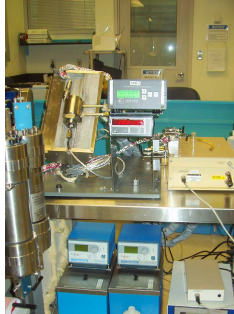
A ViscoLab PVT viscometer set up in a DBR laboratory.
