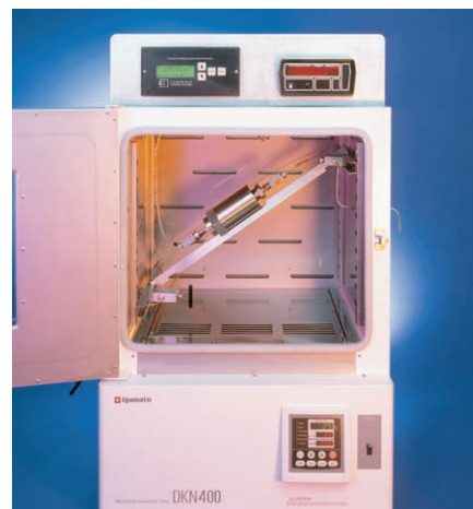
The ViscoLab PVT was an innovative instrument that made it possible to capture measurements in just a few hours, when previously they took several days.
