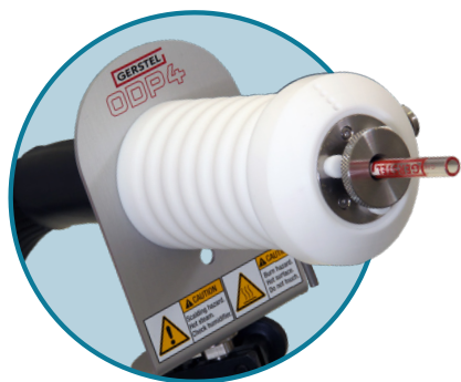
Figure 1: GERSTEL ODP 4 fitted with adsorbent tube adaptor for GC eluate collection.
