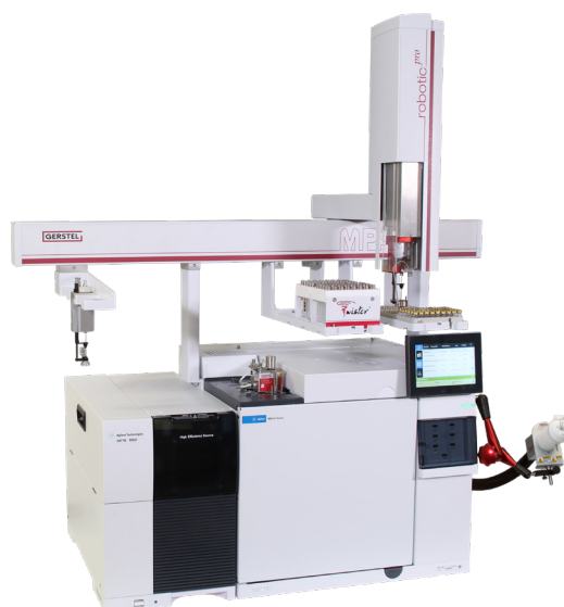
Figure 2: GERSTEL ODP 4 coupled to GC/MS system with TDU 2 and GERSTEL MPS robotic pro .
