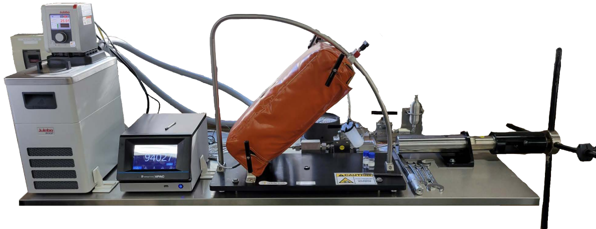
Cambridge Viscosity's ultra-high-pressure ViscoLab PVT+ system mounted on a customer's benchtop
