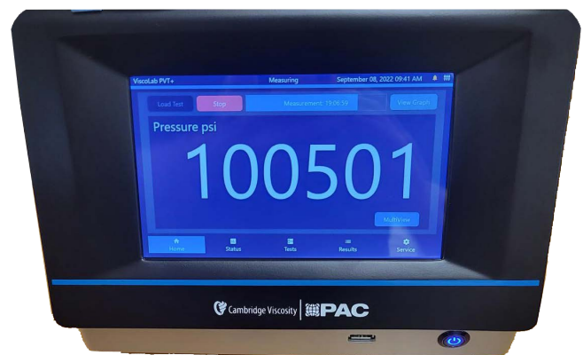
The ViscoLab PVT+ helps the end user understand how lubricants will perform under extremely high pressures.
