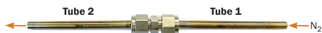
Figure 2: A pair of identical conditioned tubes connected in series for the breakthrough experiment.
