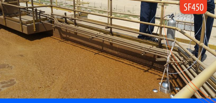
Flux Chamber designed for both solid and liquid surface sample collections.
