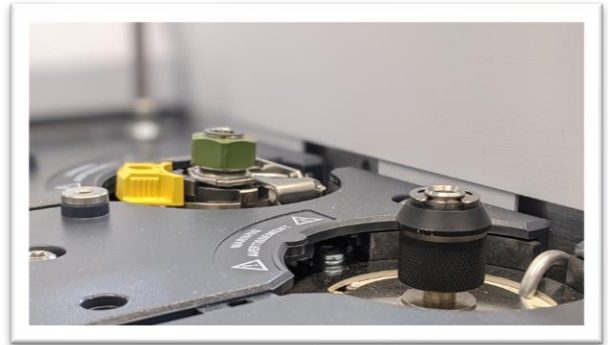
Figure 2: Split & PTV inlet on M4 prefrac.
