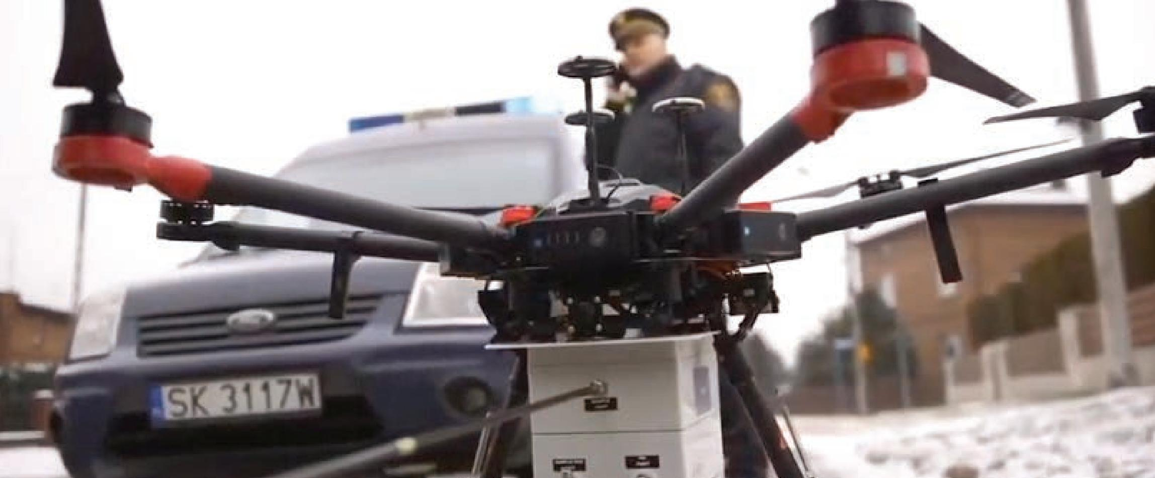
The Scentroid DR1000 flying laboratory provides continuous monitoring of multiple chemicals. While in flight, five built-in chemical sensors can provide remote monitoring of chemicals selected at the time of ordering. The Scentroid DR1000 can be used to sample and analyze ambient air at heights of up to 150 meters above ground level that was previously impossible to accomplish. Air quality mapping, model ver-
