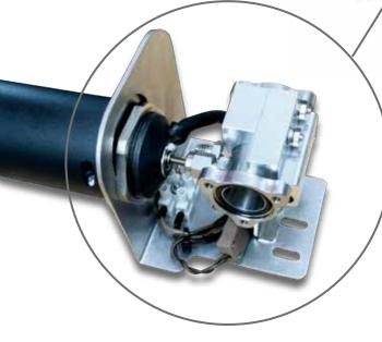
The vapors released from the material pass through a gas cell inserted in the FTIR, where the spectrum is obtained. Spectral searching provides the last link of vapors identification and thanks to the ability to detect functional groups, FTIR analysis allows greater understanding of the processes seen in the TGA.
