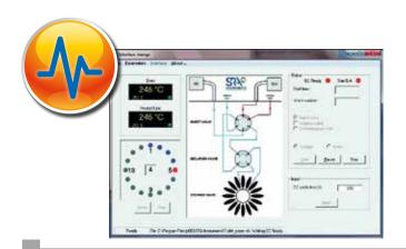
• The **SRA IST software** allows to edit the storage sequence, save the methods, view the status of the instrument and automatically manage the start of the GC analyses.
