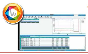
• Developed by **SRA, SOPRANE II** performs the complete management of an analysis, from the sampling to the transmission of the results. A powerful graphical environment provides effectiveness and ease of use: it is possible to define a method and a sequence of analysis, to follow the trends for specific compounds during a TGA analysis. Soprane manages the mass spectrometer and its Agilent Masshunter software and compiles all results in a same report.
