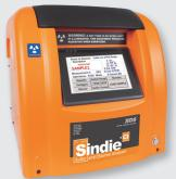
exceptional reproducibility. It delivers both sulfur and chlorine trace analysis with one push of a button and zero hassle. Samples are measured directly, which means it can analyze even the heaviest of hydrocarbons like crude oil or coker residuals, without the hassle of boats, injectors, furnaces, or changing detectors.
