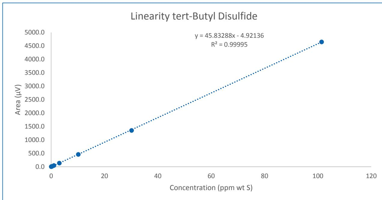
Figure 7: Linearity overlay of 30 ppb to 100 ppm tert-Butyl Disulfide
