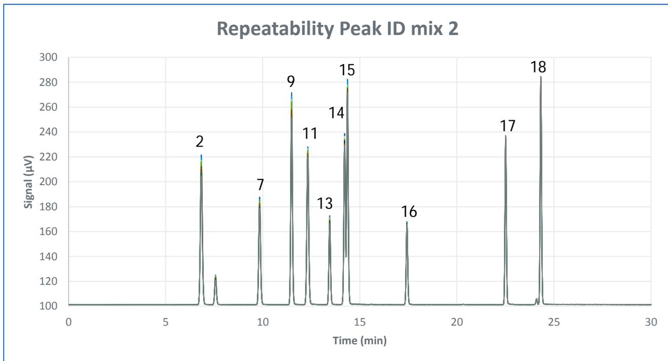
Figure 4: Repeatability overlay of 10 consecutive runs of peak ID mix 2 in ASTM D5623 ALS injection.
