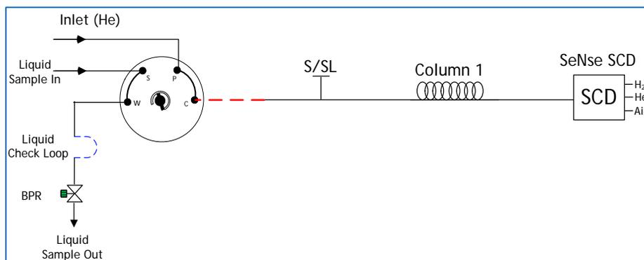
Figure 1: Plumbing diagram for Sulfur Compounds in Light Petroleum Liquids analyzer according ASTM D5623 using PAC SeNse detector (with optional LSV)
