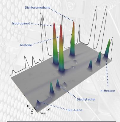
Efficient modulation of compounds <C<sub>6</sub> using INSIGHT provides sharp and symmetrical peaks for volatiles in blood.
