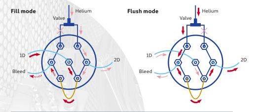
INSIGHT uses a two-stage process involving the sample loop (orange) to achieve effective modulation. In fill mode, the primary column eluate enters the sample loop (with any overfill directed to a bleed line), while the modulation valve directs auxiliary carrier gas to the secondary column. The valve then switches, and the contents of the sample loop are flushed rapidly on to the secondary column as a narrow chromatographic band.
