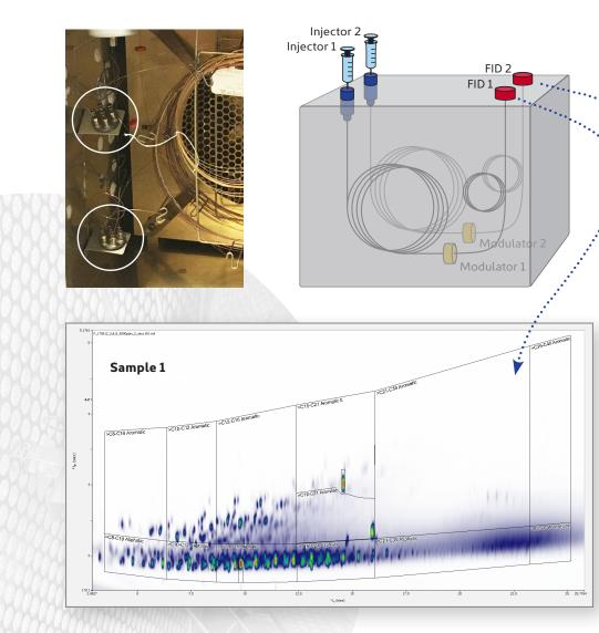
Use of two INSIGHT modulators in a dual-channel configuration immediately doubles productivity, resulting in a swift return on investment. This is illustrated for environmental monitoring of total petroleum hydrocarbons (TPH) using the 'stencil' feature in SepSolve's ChromSpace software.
