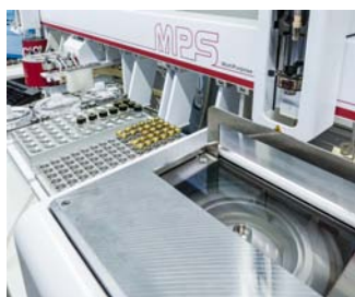
GERSTEL MultiPurpose Sampler (MPS) equipped with centrifuge, m VAP and quick Mix.
