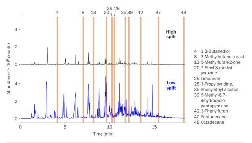
**Quantifying major and minor components from the same sample:** An initial high split of freshly ground coffee, sampled using headspace HiSorb, avoids the risk of system overload for higher-abundance components, while a lower split ratio applied to the re-collected sample (automatically retained on a clean sorbent-packed tube during the original HiSorb analysis) improves responses and allows trace-level analytes to be detected (labelled).
