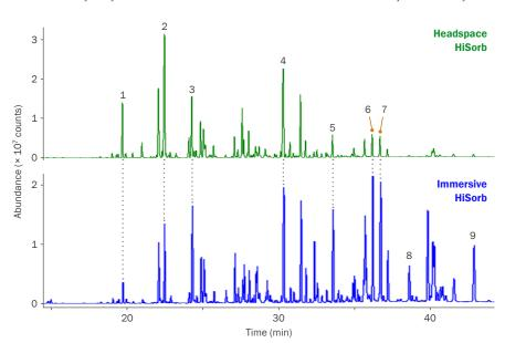
**Analysis of a fabric conditioner using different techniques** generated a more comprehensive fragrance profile. This example shows improved responses for later-eluting, less-volatile aroma-active compounds when using immersive HiSorb sampling.
