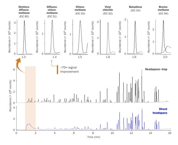
Enhanced sensitivity and excellent peak shapes are achieved, particularly for early-eluting gaseous compounds, in this 80-component mix of VOCs in water (at 20 µg/L). Sizeable improvements in the signal-to-noise ratios are obtained when combining Centri 90 with GC-MS.
