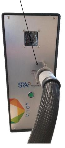
Isolate the sample line connected to the MicroGC to avoid damaging the communication cables.
