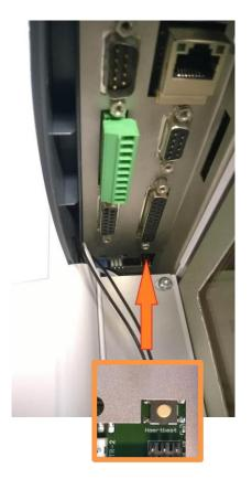
The reset button can be accessed on the main board (see pictures above). To restore the factory default IP address, follow this procedure:
