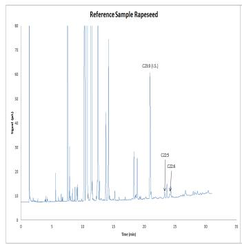
Figure 4: Reference biodiesel sample (rapeseed source). Sample contains < 0.1 % PUFA methyl ester.
