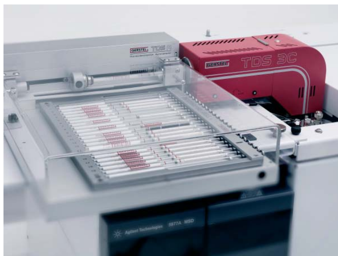
Figure 2. Thermal Desorption System (TDS 3) with autosampler (TDS A).
