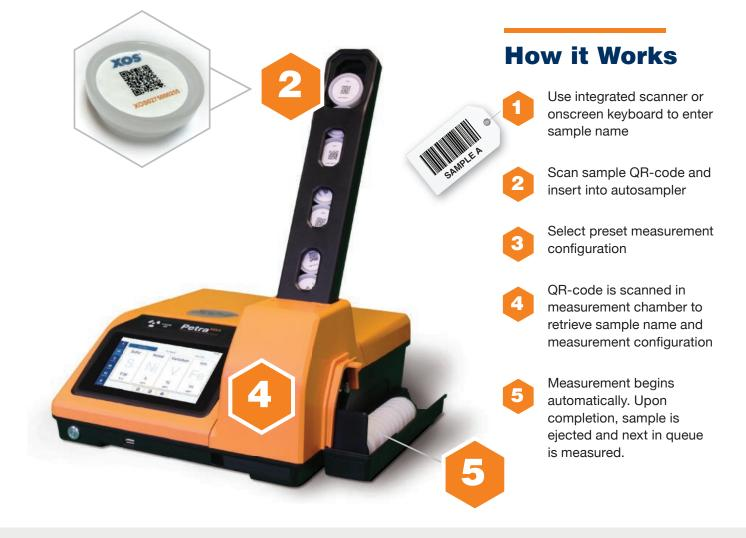
The Autosampler is an optional add-on feature, and can be added to an existing Petra 4294 or Petra MAX analyzer. QR/barcode scanner included with purchase. QR-coded cups are not mandatory - standard XRF cups may be used with the analyzer.
