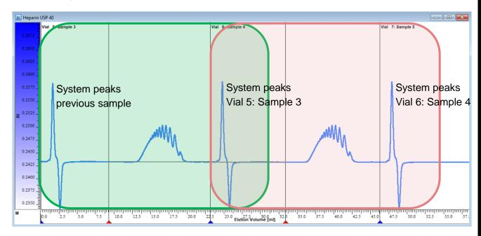
Figure 4 Overlaid injection: Vial 6 Sample 4 is injected before Vial 5: Sample 3 is completely eluted. The displayed elution volume is valid for Vial 5 sample 3, approx. 30% solvent can be saved with this software feature
