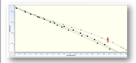
Figure 2: Overlay of different calibration curves (PS gray, PMMA black, PDMS green), measured in ethyl acetate, flow rate 1ml/min, room temperature, sample concentration 0.5mg/mL to 1mg/mL, injection volume 20µL, RI detection
