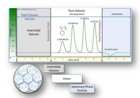
Figure 1: Graphical representation of total column volume, the interstitial volume and the pore volume of a typical analytical GPC/SEC column of the dimensions ID 8mm, length 300mm
