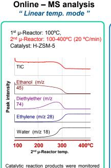
catalytic reaction products were monitored as the reaction temperature was raised at a constant rate. The amount of ethanol sharply dropped when the temperature reached 280°C, while the amount of diethyl ether increased. Also, the formation of ethylene and water is observed.
