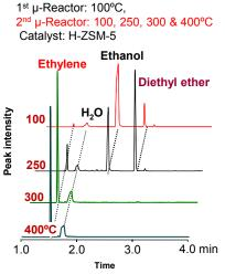
Based on the online-MS analysis results, the volatiles released from each temperature zone were introduced to a separation column and analyzed. As the reactor temperature was raised, ethylene and water were formed while the amount of ethanol formed dramatically decreased.
