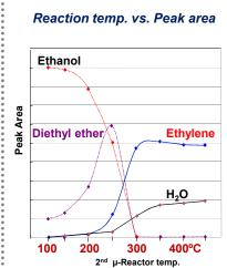
These are the plots of the peak areas obtained from the chromatogram on the left as the reactor temperature incrases. It clearly shows how the function of the ZSM-5 catalyst various with the temperature of the reactor.
