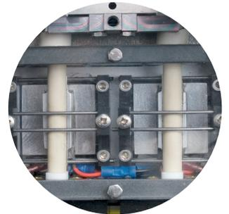
Rapid trap heating rates combined with a reverse flow of carrier gas ensure efficient desorption – giving narrow peaks and optimum sensitivity. In addition, efficient trap cooling after desorption of the sample enables the next stage of sampling to begin with the minimum of delay, making possible cycle times of as little as 3 minutes.
