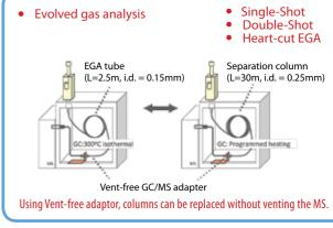
Switching between EGA tube and separation column
