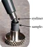
The *eyeliner* is placed directly into the sample cup and analyzed directly; there is *no sample prep*.
