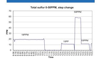
NSure can capture a significant step change within 2 sample injections (in less than 5 minutes). This demonstrates the sensitivity of this method for tracking quick changes in the process.
