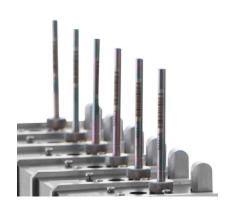
A sampling tube is attached to the outlet of each chamber, and vapours from the sample are swept onto it. The sorbent packing can be optimised for the analytes of interest.
