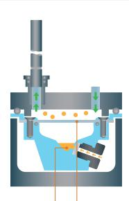
Liquid samples are injected through a septum into the well under a sealed sample of test material.
