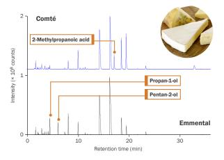
Key differences between the aroma profiles of food products are rapidly identified using the μ-CTE, as illustrated here by this comparison of vapours released from different **cheeses**.
