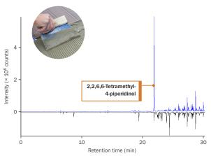
Emission profiles of similar products like these two brands of **grab-adhesive** are readily compared using the μ-CTE – aiding product development and compliance with standard methodology such as ASTM D7706-11.
