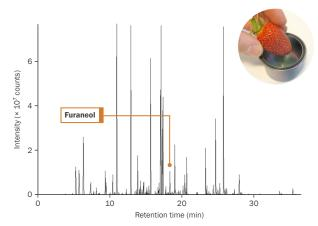
The μ-CTE is perfect for identifying target species in complex aroma profiles such as **strawberry** headspace. Furaneol was of interest in this case, with its desirable 'burnt sugar' aroma and sub-ppb odour threshold.
