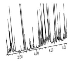
Analysis of sorbent tubes for VOCs and SVOCs uses thermal desorption (TD) with GC or GC-MS. Analysis of DNPH cartridges for formaldehyde is carried out by HPLC.
