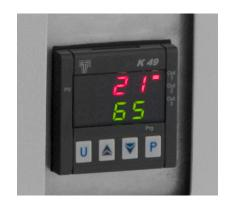
Each chamber lid is closed, a flow of gas (air or nitrogen) is applied, and the temperature selected – from ambient up to  $120\,^{\circ}\text{C}$  or  $250\,^{\circ}\text{C}$  depending on the model of  $\mu\text{-CTE}$  chosen.
