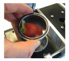
The sample is placed inside one of the chambers. Up to four or six samples can be accommodated, depending on the model of  $\mu\text{-CTE}$  chosen.
