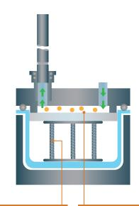
Sprung spacers raise planar samples to the top of the chamber.
