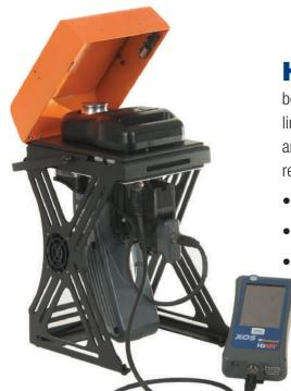
**HD Rocksand** offers much more than simple screening. With best-in-class limits of detection, HD Rocksand delivers analysis below regulatory limits – particularly for elements like Cadmium, Arsenic, and Mercury. It features an easy-to-use sample cup rotator for soil and water samples enabling improved results for heterogeneous samples.
