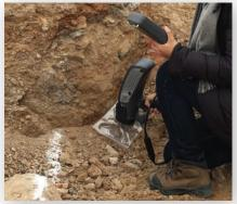
Large samples like long drill cores, pit walls, and chunks of material can be easily screened without the need to remove a sample.
