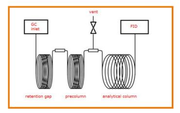
Figure Two: Column Configuration ASTM D7756
