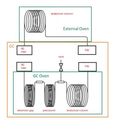
Figure Three: Column Configuration ASTM D7756 & D2163
