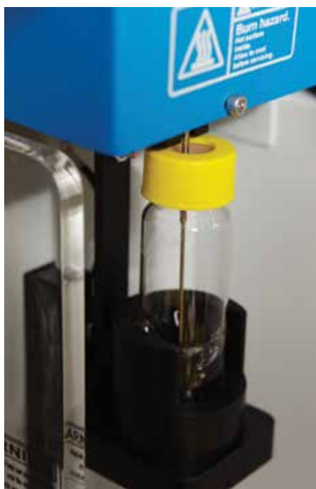
Samples run in the soil position can be heated and stirred while being purged
