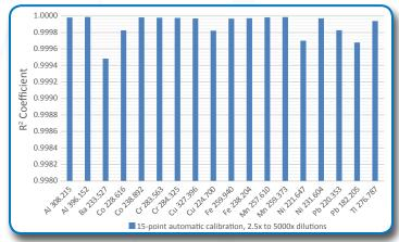
Automated calibrations on ICP using a 1000 ppm multielement standard solution produced R<sup>2</sup> values greater than 0.999 for elements measured. Curves contained fifteen calibration points with dilutions between 2½:1 and 5000:1.
