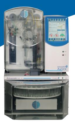
The Aurora 1030C employs high temperature (680 °C) catalytic combustion to oxidize and convert organic compounds present in aqueous samples to  $CO_2$  for measurement by a solid state non-dispersive infrared (SS-NDIR) detector.
