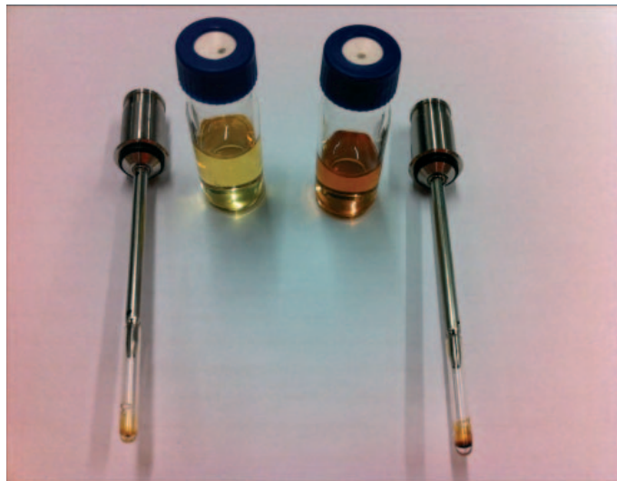
Figure 1a. QA whiskey (left) and QR whiskey (right) together with QA residue in pyrolysis sample holder (left) and QR whiskey residue in pyrolysis sample holder (right).
