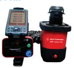
FlexScan analyzer uses the same interferometer and optics as the 4100 ExoScan FTIR and thus has identical performance. The 4200 FlexScan is for dedicated field applications and has a fixed sampling interface that is specified when the system is ordered. The light weight of the handheld optics and sampling module make it well suited to repetitive infrared analyses over a large area.
