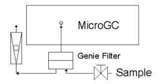
If there is a risk of condensation of the sample (organic solvents or high-boiling compounds), it is preferable to choose the same system installed in a heated and insulated box.
