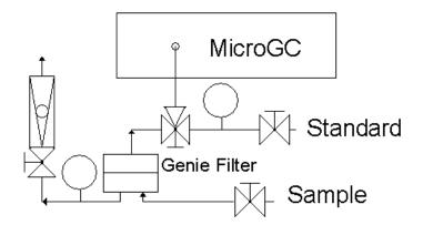
In the figure above, the standard and sample are connected to a 3-way valve that can be automated. The sample is still circulating but the standard is retained and used only for calibration.
