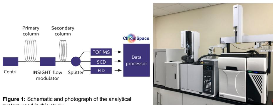
Figure 1: Schematic and photograph of the analytical system used in this study.
