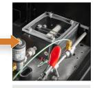
The trap is thermally desorbed at up to 100°C/s to inject the sample into the GC-MS as a narrow band.
