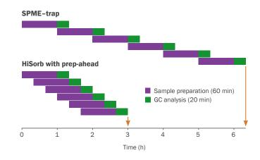
**By using a 'prep-ahead' workflow**, six HiSorb samples can be run in less than half the time of six SPME or SPME-trap analyses.
