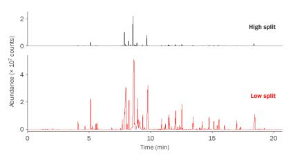
**Re-collection allows multiple methods to be applied to the same sample:** In this example, an initial high split of a candle wax sample avoids the risk of system overload, while a lower split ratio on the re-collected sample allows trace-level components to be detected.
