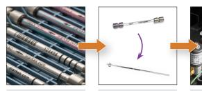
Capped tubes are placed in trays and leak-tested to confirm sample integrity, as required by standard methods. Analytes are releasedThefrom the tubes in adesflow of heated gas,100and the vapourssamcollected on theGC-focusing trap.ban
