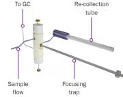
Field-proven over 20 years, it is this proprietary valve-trap combination that allows Centri to offer selective purging of water to vent and accommodate analytes over a wide volatility range. It also delivers features that are essential for enhanced data confidence, such as stringent pre-analysis leak-checking, and the option of internal standard addition before each run.
