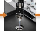
The probe is removed from the vial, and a wash/dry station removes residual sample matrix.
