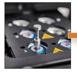
The robot inserts the probe into the vial, and the assembly is incubated/agitated to ensure analyte equilibration.
