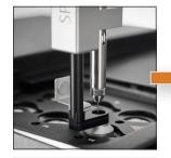
The SPME fiber is normally positioned in the sample headspace and incubated/agitated to facilitate extraction.
