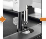
The fiber is inserted into the injection port and the vapours transferred to the focusing trap (or sent directly to the GC–MS).
