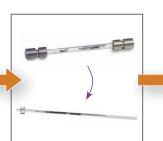
Analytes are released from the tubes in a flow of heated gas, and the vapours collected on the focusing trap.
