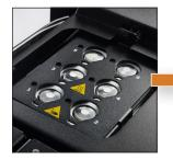
The sample vial is incubated/agitated to speed up analyte equilibration.
