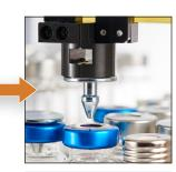
The headspace vials are re-sealed with special caps to avoid contamination of laboratory air.
