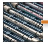
Capped tubes are placed in trays and leak-tested to confirm sample integrity, as required by standard methods.
