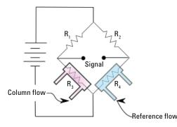
Figure 1. Schematic overview of a thermal conductivity detector.
