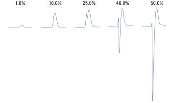
Figure 2. Peak shape of increasing hydrogen concentrations with helium carrier gas.
