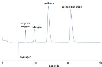
Figure 3. Chromatogram for permanent gas analysis on MolSieve 5A column, including negative hydrogen peak, using mixed carrier gas.
