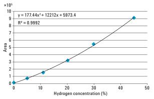
*Figure 6. Calibration curve (quadratic fit) for hydrogen using 8.5% H*<sub>2</sub> *in He carrier gas.*
