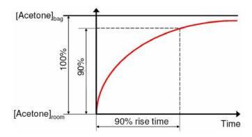
Figure 1. Illustration of the response to a step change in acetone concentration at the inlet of the SIFT-MS instrument. The measured concentration rises more slowly than the actual concentration presented to the instrument's inlet due to the dynamic response characteristics of the analyzer. The 90% response time should be  $\leq 10\%$  of the duration of an exhalation to accurately measure end-tidal concentration.
