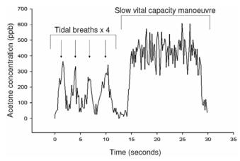
Figure 2. Example of detection of acetone during four tidal breaths then a slow vital capacity maneuver via the mouth.
