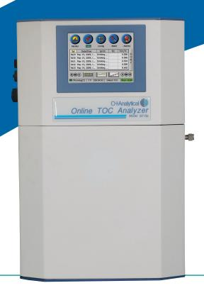
The OI Analytical 9210p On-line Total Organic Carbon (TOC) Analyzer is designed to continuously monitor TOC levels in process water streams. The 9210p uses proven heated persulfate oxidation technology for accurate, dependable operation and regulatory compliance. Virtually all organic compounds dissolved in water can be oxidized with high efficiency by this technique.
