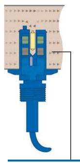
The robust Cambridge Viscosity oscillating piston system can measure a wide range of samples, including asphalt, lubrication oils, and heavy fuel oils, as well as handle any process upsets without damage to the system.
