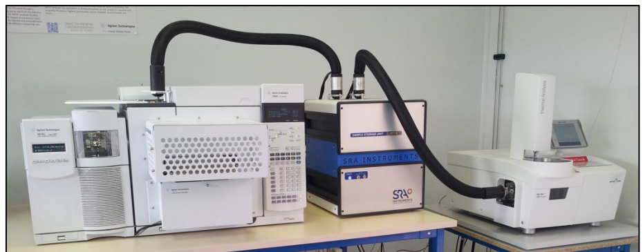
Fig.3: IST interface (center) coupled with Agilent GC/MS (left) and METTLER TOLEDO TGA/DSC 1 (right)
