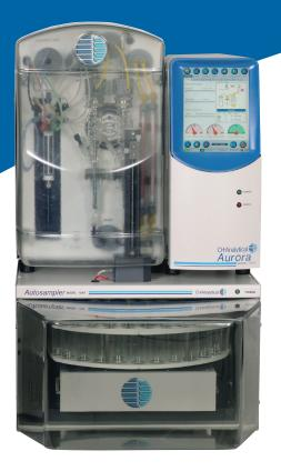
The Aurora 1030W Total Organic Carbon (TOC) Analyzer uses the proven heated persulfate wet oxidation technique to analyze organic contamination levels in aqueous samples. Virtually all organic compounds dissolved in water can be oxidized by heated sodium persulfate ( $Na_2S_20_8$ ). Concentrated solutions (1 or 1.5 M) can effectively oxidize organic matter present in the form of colloids, macromolecules, and suspended solids.
