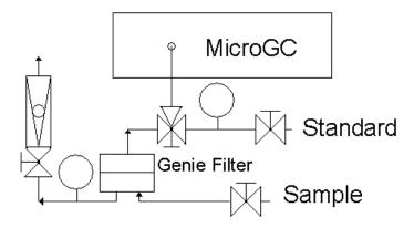
In the figure above, the standard and sample are connected to a 3-way valve that can be automated. The sample is still circulating but the standard is retained and used only for calibration.
